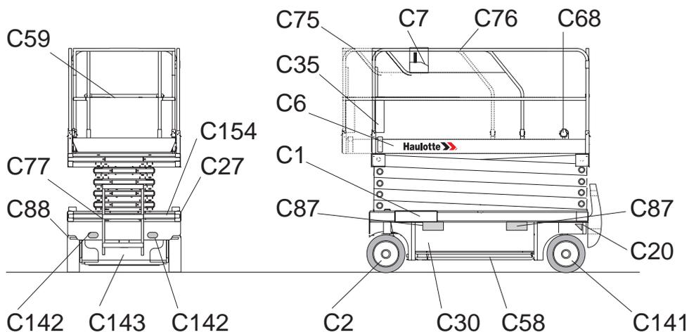
OPTIMUM 6 (OPTIMUM 1530E) - OPTIMUM 8 (OPTIMUM 1930E) - Vista dos componentes
